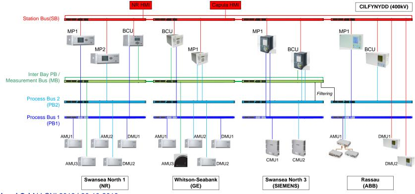
• VSATT has enabled NG to proceed with the first Process Bus (PB) applications, i.e. PMU
